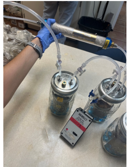
Top Left: Closed survey chamber connected to a drierite trap and metal canister for surface soil gas sample collection in the field.
