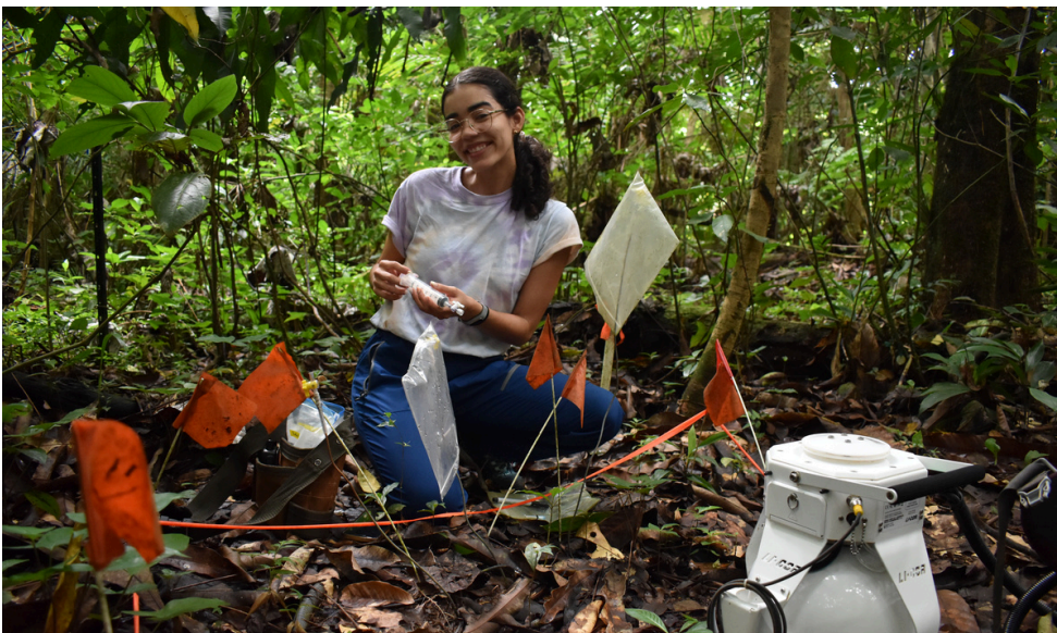
Top Left: Closed survey chamber connected to a drierite trap and metal canister for surface soil gas sample collection in the field.
