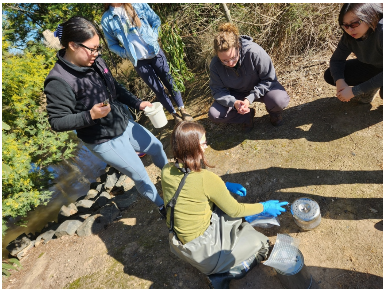
Figure 2: Francesca Ferguson teaching Penn State undergraduate and Monash collaborators how to deploy a Polar Organic Chemical Integrative Sampler to investigate emerging contaminant concentrations in the Gippsland Watershed.
