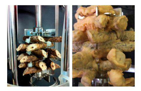
Integral to the ability of biofilm reactors to produce vitamin K are specially designed internal plastic composite supports that microorganisms adhere to and build intertwined colonies – called biofilms – that can withstand aeration and agitation needed to spur the microorganisms to secrete more vitamin K. These photos show the supports before fermentation (left) and covered by biofilms. **IMAGE: EHSAN MAHDINIA / PENN STATE**
